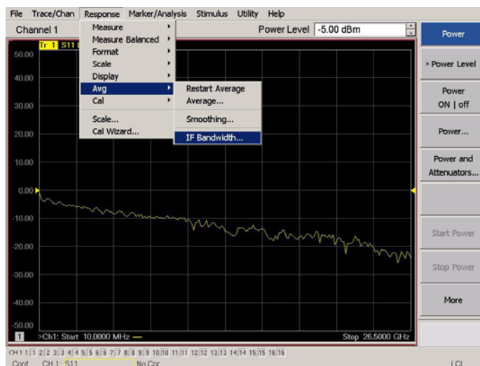
Figure 46 Setting the IF Bandwidth
